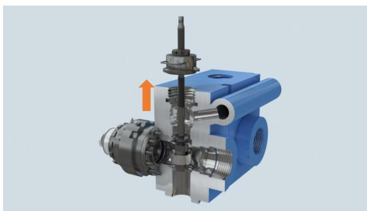
► Remover the bolt, cylinder, cylinder seat. Remove the puller rod.
